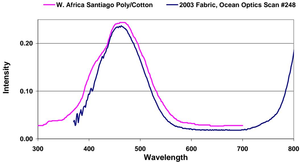
The “New Blue” VF fabrics from 2003 are a good imitation of the colour phthalogen blue on cotton and are also very similar to the Santiago poly/cot, and the Klopman “New Azzurro” poly/cot. Below is a comparison of the digitized spectrum and a spectrum taken from the actual fabric with the Ocean Optics spectrophotometer.
