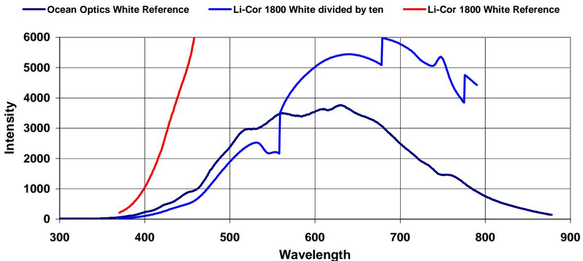
Below is a typical example of the raw signal to noise ratio (white to dark) for the two devices. The rapidly dropping ratio below about 420 nm for the Ocean Optics device is why caution should be used when interpreting ultraviolet readings from this simple device.
