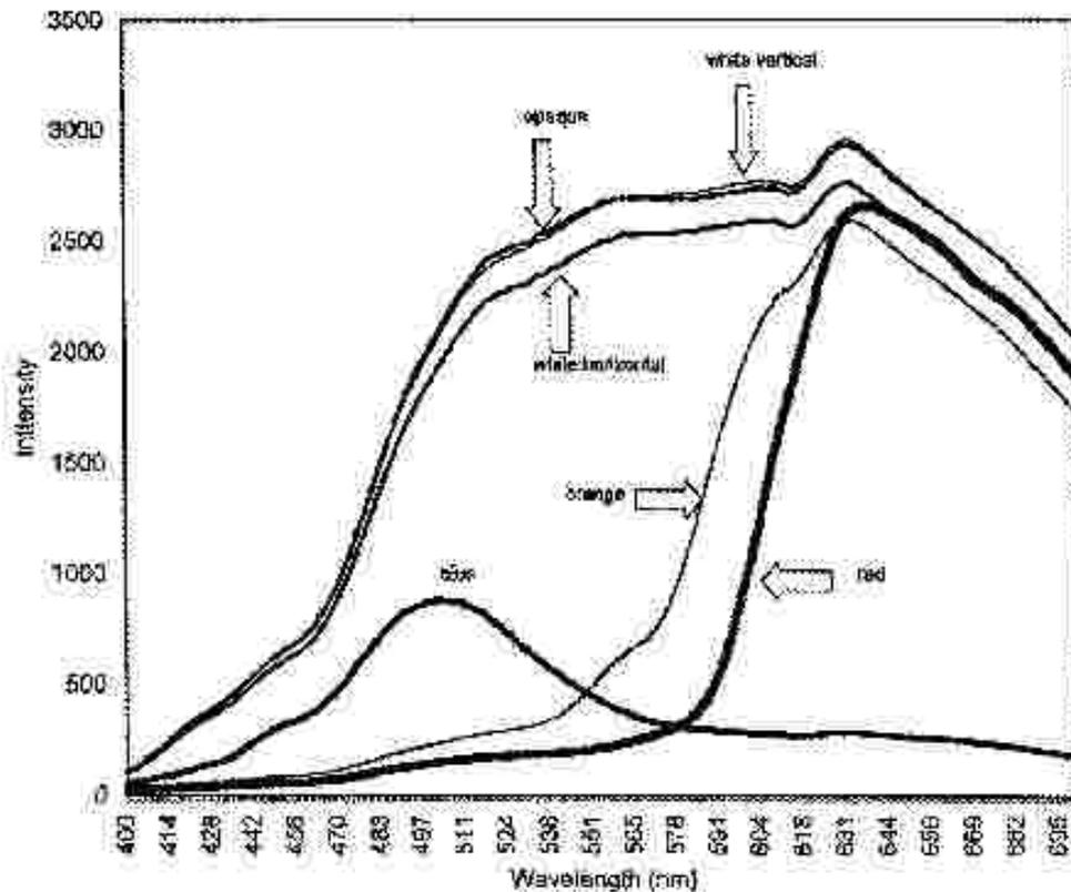
Fig 1 Spectral reflectance curves of various colors and type of plasticized corrugated boards.
