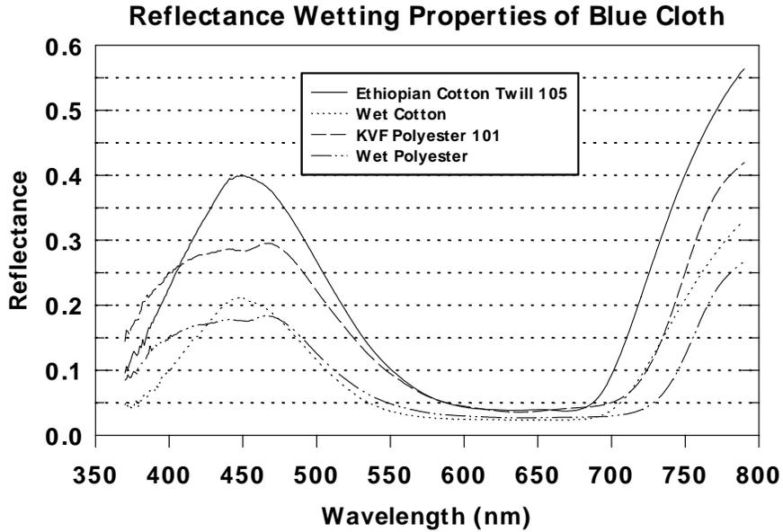
**Phthalogen blue cotton is nearly opaque when dry (5% transmittance). When wet, transmittance changes to 20%, a much larger change than for a similar blue polyester.**
